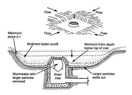
Fig. 16 – Sediment trap
