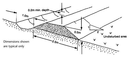
Fig. 11 - Bank with drain
