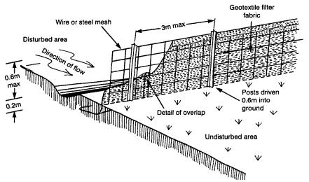
Fig. 15 – Typical sediment fence
