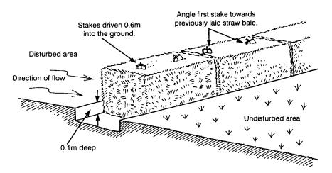
Fig. 14 – Straw bale sediment filter
