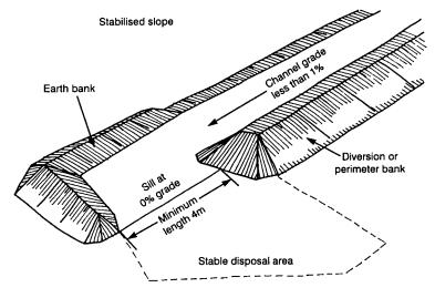
Fig. 13 - A level spreader or sill
