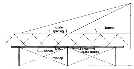
Fig. 1 – Mobile boom irrigation provides even, light (e.g. 5 mm/hr) applications of water which are ideal for plugs and flats
