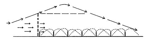
Fig. 4 – A well designed artificial windbreak can protect sprinkler water patterns
