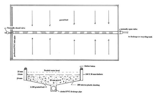
Fig. 7 - Arrangement of gravel flood floor system
