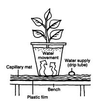
Fig. 9 – Capillary matting efficiently moves water into containers
