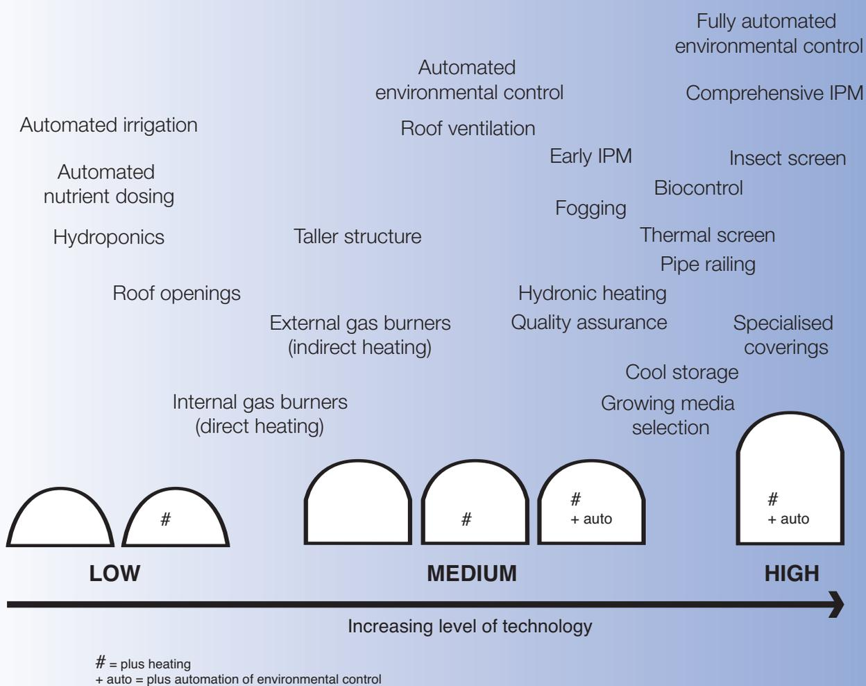
Increased levels of technology in a greenhouse provide greater environmental controls
